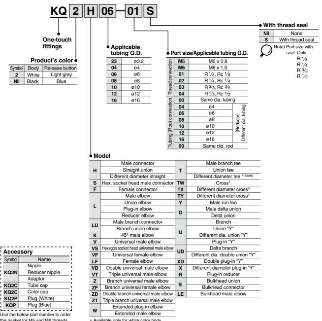
the gasket for M5 and M6 threads. Gasket for M5 thread: M-5G2 Gasket for M6 thread: M-6G
